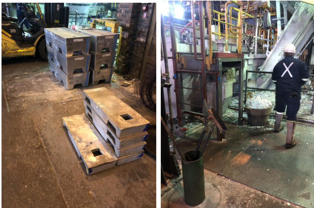
Zinc is added to the process and zinc dross is skimmed off manually.
